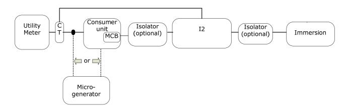
Use solid core cable between the I2 and the MCB suitable for >16amps, such as at least 2.5mm2 twin and earth. Follow IEE wiring standards. Between the I2 and the load 2.5mm2 or 4mm2 twin and earth may be needed for a 3kW load. The terminals accept up to 4mm2.
